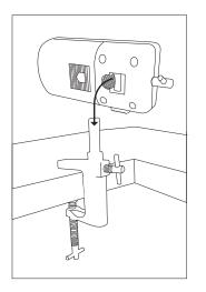
2. Twist the T-screw on the magnifier to tighten on C-clamp as shown below. Magnifier will be able to rotate 360°.
