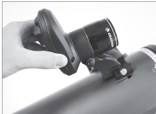
Installing small base (back to front)
