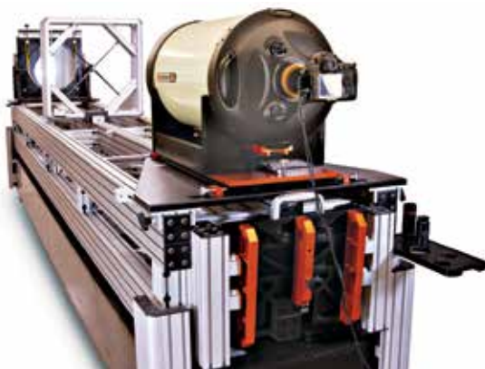
FIGURE 12. In the Final Acceptance Test, the EdgeHD optics must demonstrate the ability to form sharp images at the center and in the corners of a full-frame digital SLR camera, with a sensor that measures 42mm corner-to-corner.
