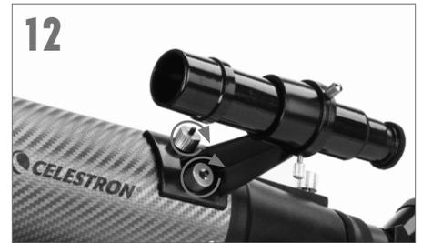
Locate the finderscope and remove the plastic caps on the front and back lens. Orient the finderscope so that the larger lens is facing towards the front of the tube as shown. Place the finderscope over the posts on the tube and replace the knurled nuts to secure it in place.
