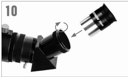
Insert the barrel of the 20mm eyepiece into the diagonal and tighten the set screw.
