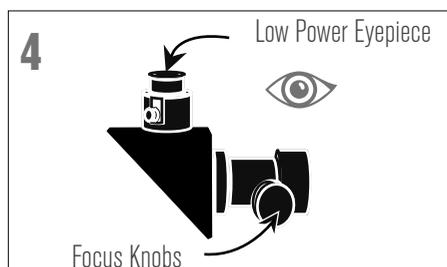
4 Look through the telescope's 20mm eyepiece. Gently turn the focus knobs to adjust the sharpness of the image.
