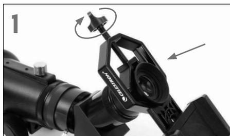
1 Open the eyepiece clamp and place it around the body of the eyepiece. Tighten the clamp until it's secure.
