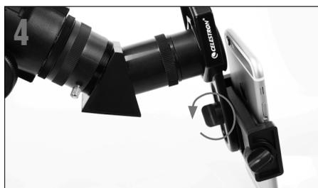
4 Loosen the knob on the bottom of the adapter that secures the phone clamp to the eyepiece clamp. Slide the phone clamp up and down and rotate it left and right until your camera is looking down through the eyepiece of the telescope. Tighten the knob on the bottom of the adapter to secure it in place.
