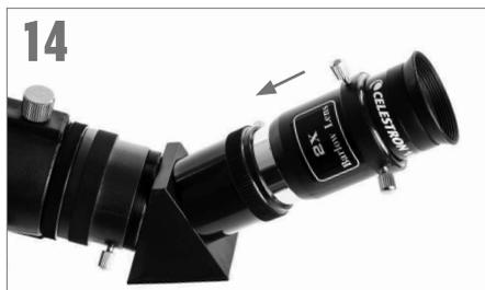
For additional magnification, you can use the included 2x Barlow lens. Place the Barlow lens between the diagonal and the eyepiece.
