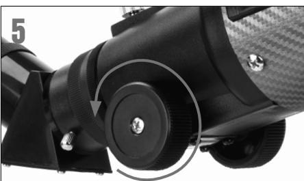
5 Use the telescope's focuser to adjust focus of your camera. Snap the image using your app.
