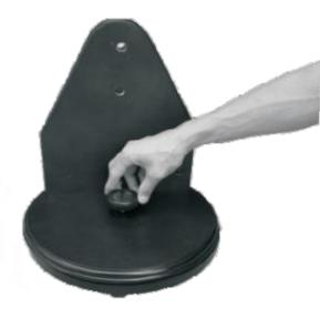
9.(1) REMOVE LOCKING KNOB, WASHER AND SLEEVE FROM BOLT (ON THE HUB OF THE TUBE)
