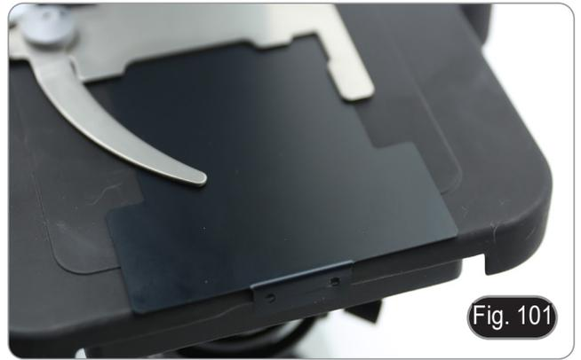
Mode n° 2: lower the condenser and insert the plate between the two layers of the stage. (Fig. 102)
