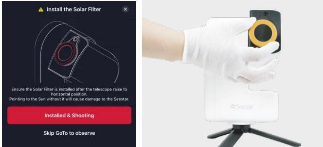
To ensure maximum safety for both you and the device, auto GOTO will stop once the lens roughly points at the Sun. Follow the App's instructions and manually adjust the lens to point directly at the Sun.
