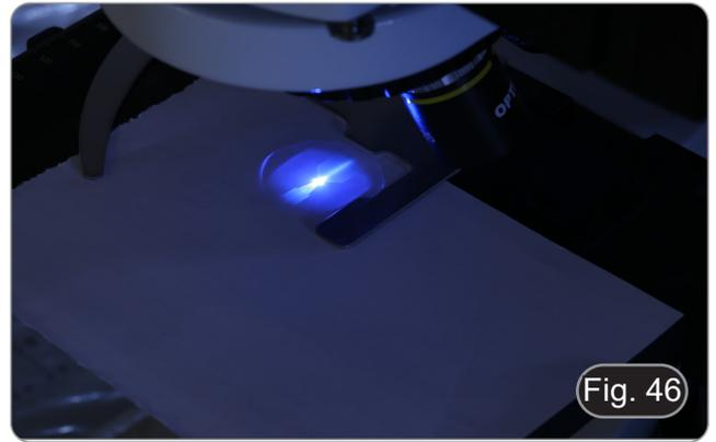
7. Using the focusing screw of the collector lens ② enlarge the image until a homogeneous illumination is achieved (Fig. 47). At this point, insert an objective into the optical path and, looking into the eyepieces, optimize the illumination always using the screws ② and ③.
