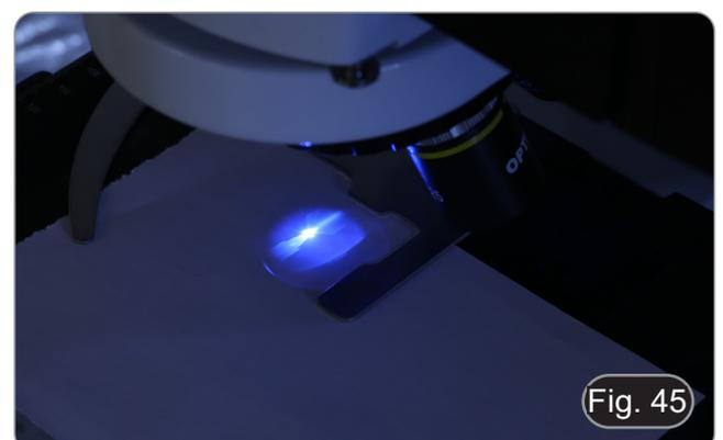
6. Using the centering screws ③ on the side of the lamp housing, center the image of the arc. (Fig. 45-46)
