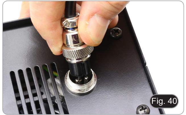
5. Insert the power cord into the connector ⑤. (Fig. 41)
