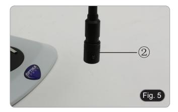
1. Move the terminal part downwards to have a more concentrated light beam. (Fig. 6)
